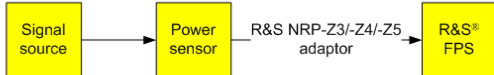
Fig. 5-2: Power sensor support – standard test setup
